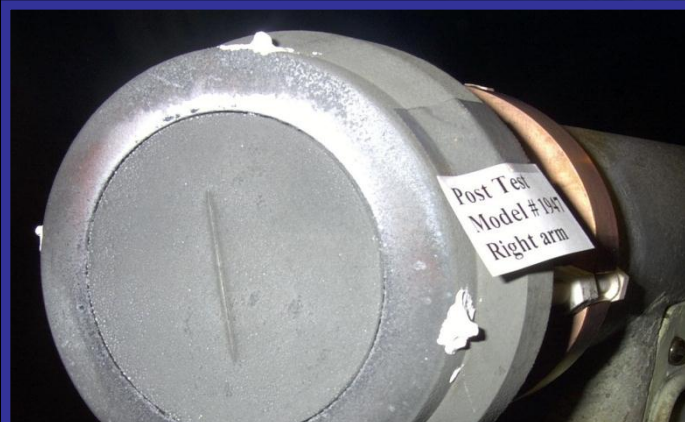
Frontside Post-Test View of 0.007 inch Slot at 2800F & 100 psf
