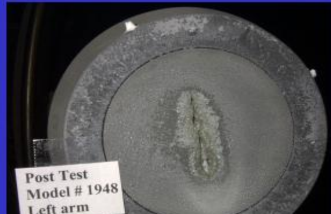
Frontside Post-Test View of 0.007 inch Slot at 3000F & 148 psf
