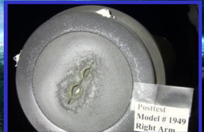
Frontside Post-Test View of 0.015 Slot at 3000F & 148 psf
