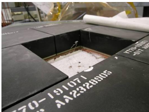
Missing Tile Damage
