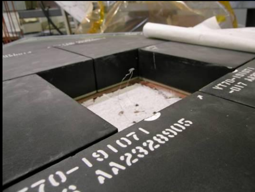
Missing Tile Damage
