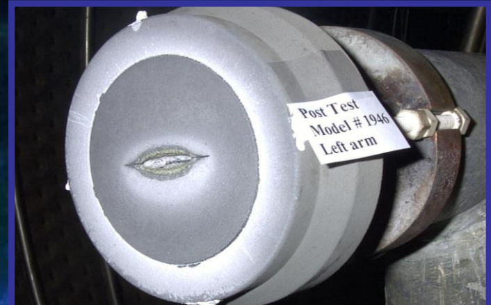
Frontside Post-Test View of 0.015 inch Slot at 2800F & 100 psf
